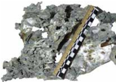
| (Fig. 13.2) — Frontal flak damage to an engine cover (P. Murphy © WWIIBRPG).
