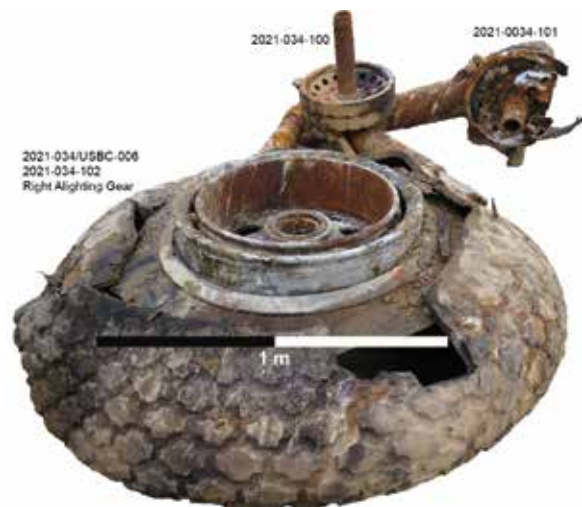
(Fig. 5.3) — Left wheel/tire and main landing struts of right and left aligning gear from Bull Session, USBC-006 (Photo P. Murphy © WWIIBRPG).
