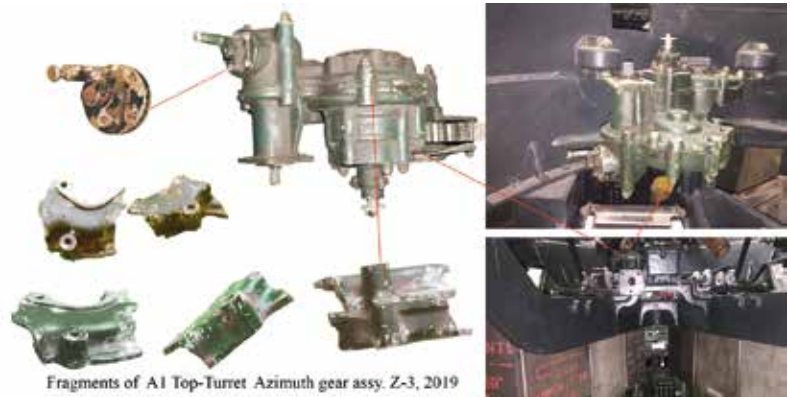
(Fig. 7.1) — left, the fragments found are from the upper turret azimuth gear housing from the Weicherdange site of Sneakin Deacon. The photo right (David Littleton image) is the azimuth gear in position inside the upper turret trunnion ring; elevation gear has a similar housing but differs in mounting and size/shape (Photo montage P. Murphy © WWIIBRPG).
