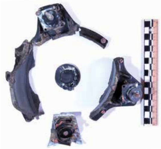
(Fig. 15.1) ____ Flux Gate Gyro transmitter- Bendix Corp located in the left wing.
